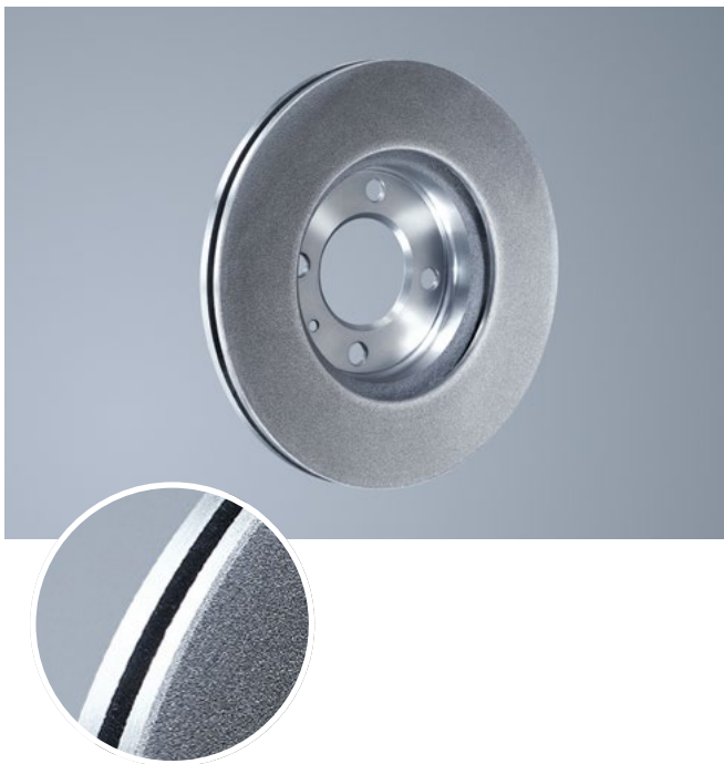
Cross section of a brake disc coated with HS-LMD with carbides embedded in a stainless steel matrix (here: TiCFeCr).
